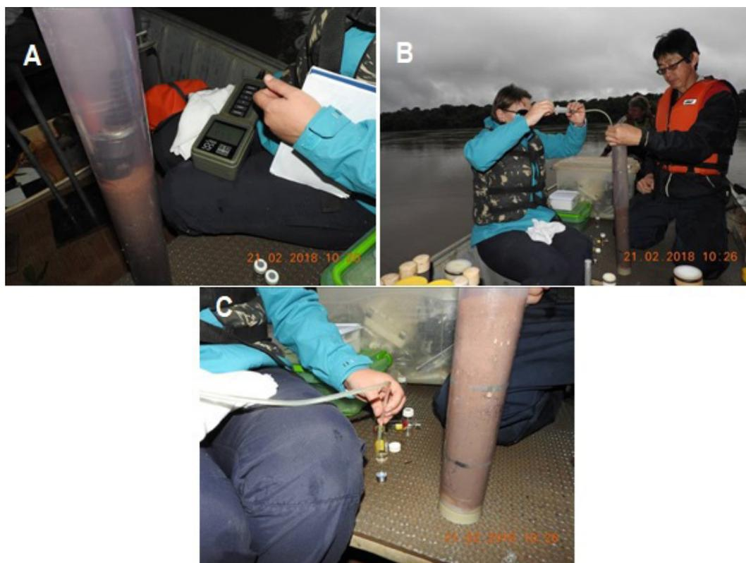
**Figure 4.** Photographic record of the quantification of temperature and dissolved oxygen (A) and the collection of water samples (B and C) for the quantification of CO<sub>2</sub> in the layer above the sediment-water interface in the sediment core collected in the future reservoir of UHE Sinop. Source: AIIEGA (2018).
