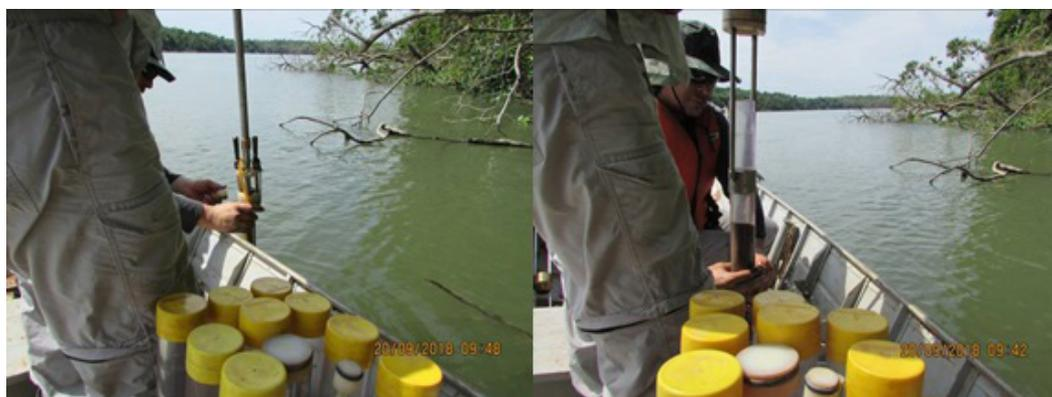
**Figure 3.** Photographic record of sediment sample collection in the future reservoir of HPP Sinop with the aid of a telescopic manual rod coupled to the Kajak-Brinkhurst type witness. Source: AIIEGA (2018).
