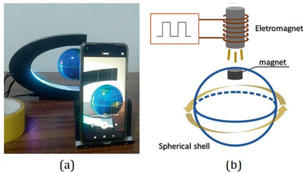
**Figure 1:** Experimental apparatus – rotary floating sphere in the air. (a) Picture of apparatus. (b) Schematic representation (not to scale). The resistance air force is only caused by skin friction, there is no contribution of pressure drag as in the translation motion.
