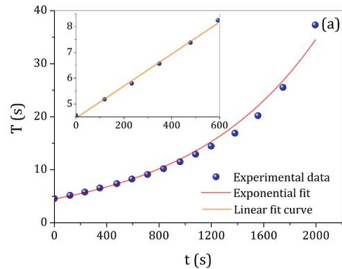
**Figure 2:** The graph shows the experimental data (circles) and two fitted curves (line) for the relationship between the period of rotation  $T$  of the levitating sphere and the elapsed time  $t$ . In general, points obey  $T \propto \exp(at)$  behavior, where  $a > 0$  is a constant. The inset illustrates that the linear function,  $T \propto t$ , is a special case as  $t \rightarrow 0$ .
