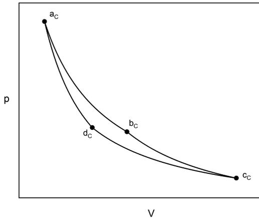
**Figure 1:** Schematic view of a Carnot Cycle. The processes  $a_C \rightarrow b_C$  and  $c_C \rightarrow d_C$  are isothermal transformations. The processes  $b_C \rightarrow c_C$  and  $d_C \rightarrow a_C$  are adiabatic transformations.
