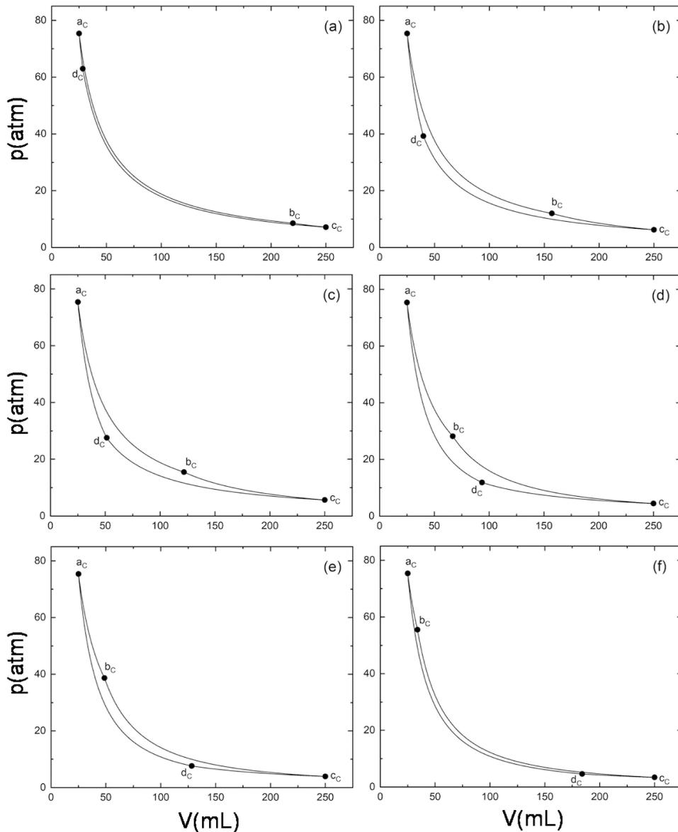
**Figure 2:** Examples of Carnot cycles of same compression ratio  $r_{V_C} = 10$ , working gas with  $\gamma = 1.4$  and different efficiencies  $e_C$ . The efficiencies are (a)  $e_C = 0.05$ , (b)  $e_C = 0.17$ , (c)  $e_C = 0.25$ , (d)  $e_C = 0.41$ , (e)  $e_C = 0.48$  and (f)  $e_C = 0.55$ .
