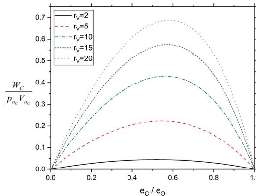
**Figure 4:** Work per Carnot cycles  $W_C$  in units of the highest energy state  $p_{a_C} V_{a_C}$  varying with the efficiency for some values of  $r_V$  (distinguished in the legend). The working gas  $\gamma = 1.4$  is the same for all cycles.
