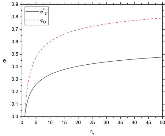
**Figure 5:** Carnot Cycle efficiencies  $e_C^*$  (solid line) that give a maximum work depending on  $r_V$  values considering  $\gamma = 1.4$ . In comparison, we depicted the Otto cycle efficiencies  $e_O$  (dashed line) relative to  $r_V$  values.
