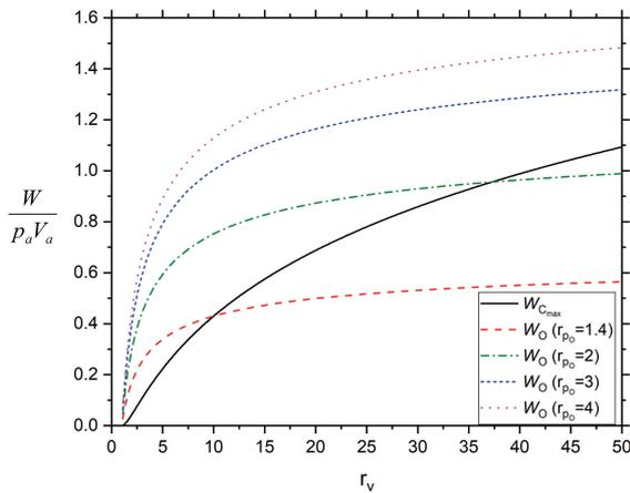
**Figure 6:** Maximum work per Carnot cycles  $W_{C_{max}}$  (solid line) for different compression ratios  $r_V$ . In comparison, we plot the work per Otto cycles (lines distinguished in the legend) dependence on  $r_V$  for different pressure ratios  $r_{pO}$ . Work values are expressed in units of the highest energy state  $p_{aC} V_{aC}$ . The working gas  $\gamma = 1.4$  is the same for all cycles.
