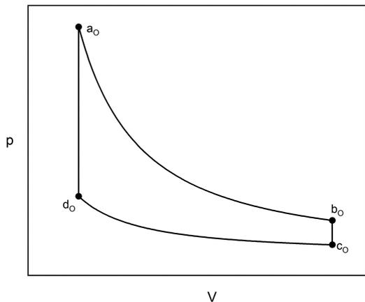
**Figure 3:** Schematic view of an Otto Cycle. The processes  $a_O \rightarrow b_O$  and  $c_O \rightarrow d_O$  are adiabatic transformations. The processes  $b_O \rightarrow c_O$  and  $d_O \rightarrow a_O$  are isochoric transformations.
