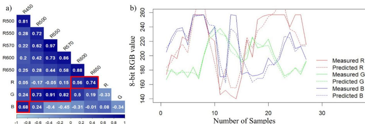
Figure 4. AS7262 spectral variables (a) related to RGB values (b) measured and predicted from 27 samples with linear regression.
