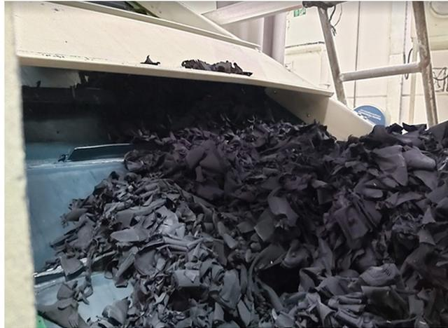
**Figure 1:** Recycling of the single jersey fabric scraps in the rag puller machine.
