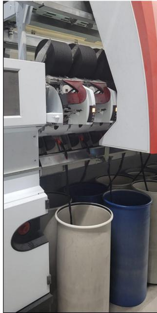
Figure 3: Recycled fiber was spun into yarn on the Saurer Autocoro 8 open-end spinning machine.
