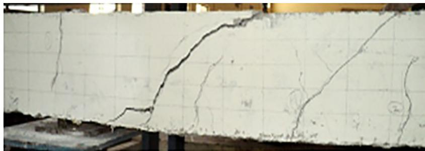
**Figure 9:** Pattern of beam B1a failure.
