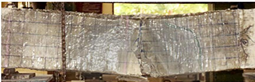
Figure 11: Pattern of beam GB1 failure.
