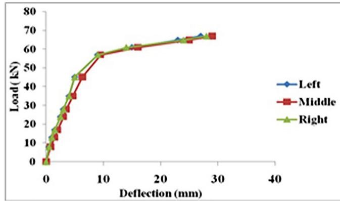
Figure 10: Curve of load versus deflection for beam GB1.
